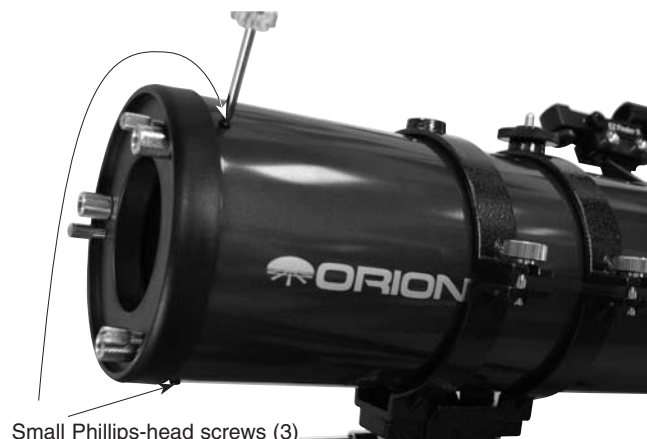
Figure 10. To remove the mirror cell from the telescope, the three small Phillips-head screws on the perimeter of the mirror cell must be completely unthreaded.
