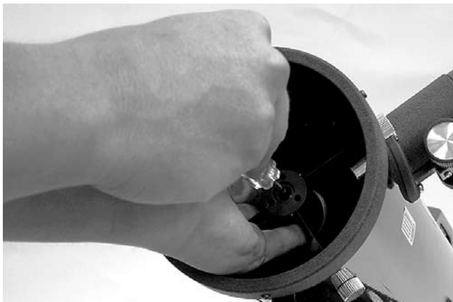
Figure 5. To center the secondary mirror under the focuser, hold the secondary mirror holder in place with your fingers while adjusting the center screw with the Phillips head screwdriver. Do not touch the mirror's surface.
