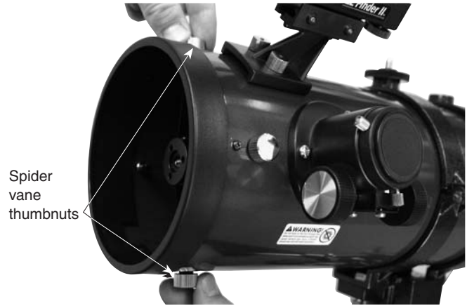
Figure 6. To center the secondary mirror up-and-down in the focuser drawtube, make adjustments to the two knurled spider vane thumbnuts that are perpendicular to the focuser.
